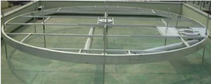
Test IFR at our factory. Note that the pontoons are not connected to the landing legs.
