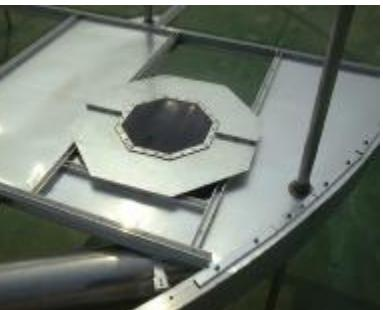
Column seal assembly (above) and standard 600mm deck Manway (left). 310mm deep extruded rim (below) is strong enough for the BTE IFR shoe seal to be connected to it without additional bracing
