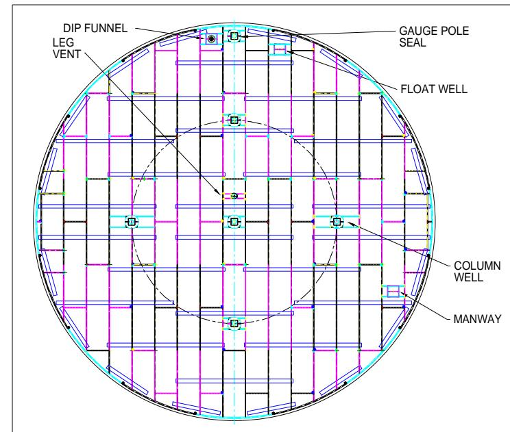
All major IFRs components are designed to pass through a 24" diameter manway, and are pre-cut for easy on-site assembly. IFRs are usually shipped in 20ft or 40ft containers.
