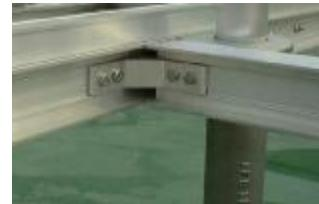
Pontoons are not connected to the landing legs. Pontoons are connected to the main frame and are unaffected by IFR flexing
